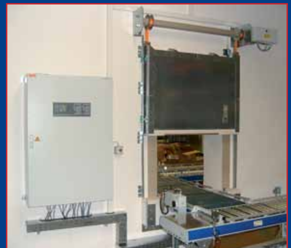
Continuous belt conveyor with 400 V emergency power system
