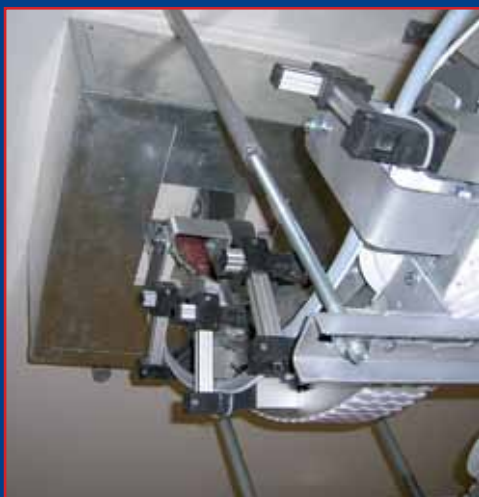
Hinge chain conveyor through ceiling openings
