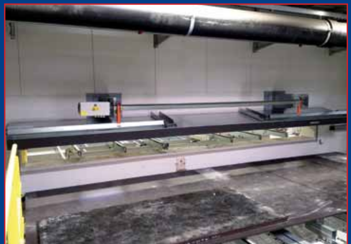
Continuous special conveyor (5 m width)
